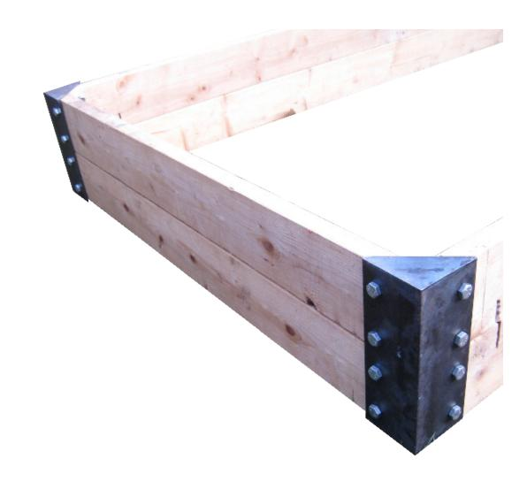
These steel corner brackets were designed to provide a simple solution to raised garden bed construction. The brackets are constructed from 1/4" steel plate and attach to 2"x6" lumber with a series of stainless steel 1/2" bolts or lag screws.
